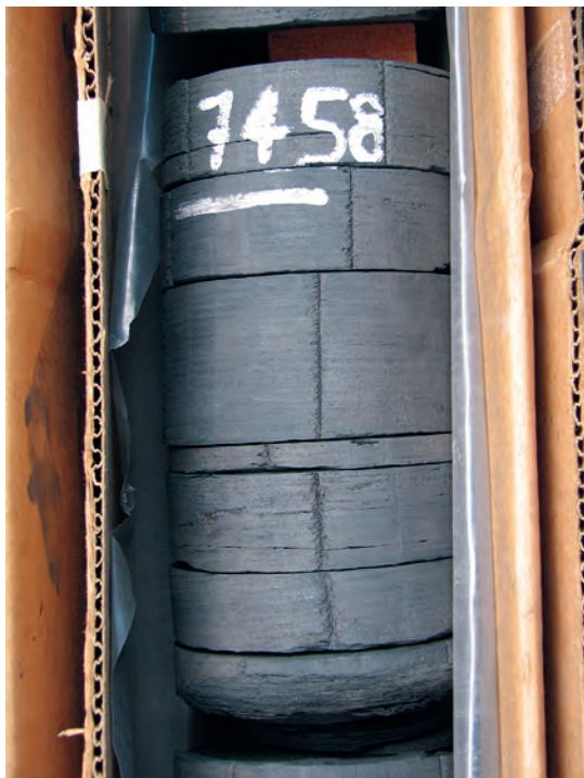
Figure 28. (Left) basal contact at 7,499.4 feet of calcareous black shale with the underlying limestone and gray calcareous shale of the Onondaga Limestone; (right) black, sooty, organic-rich Marcellus Shale; (bottom) close-up of organic-rich shale, MERC-1, Monongalia County, West Virginia.
